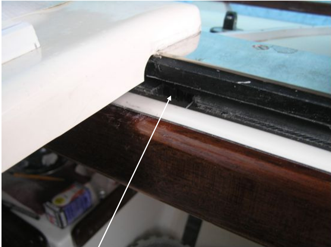
Plastic runners – note lower edge of groove cut away just in front of garage
