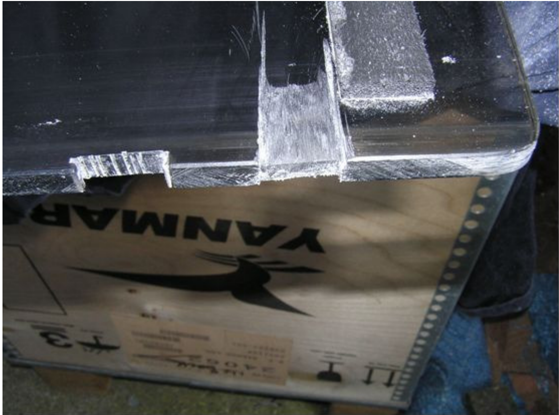
Filing chamfered slot in front of sealing strip
